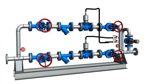
The design normally includes isolation valves installed on the upstream and downstream side of the station on each stream (Four valves), two strainers, two pressure regulating valves, two drain ball valves, two pressure gauges with ball valves, two hose isolation ball valve and one surge relief valve.
